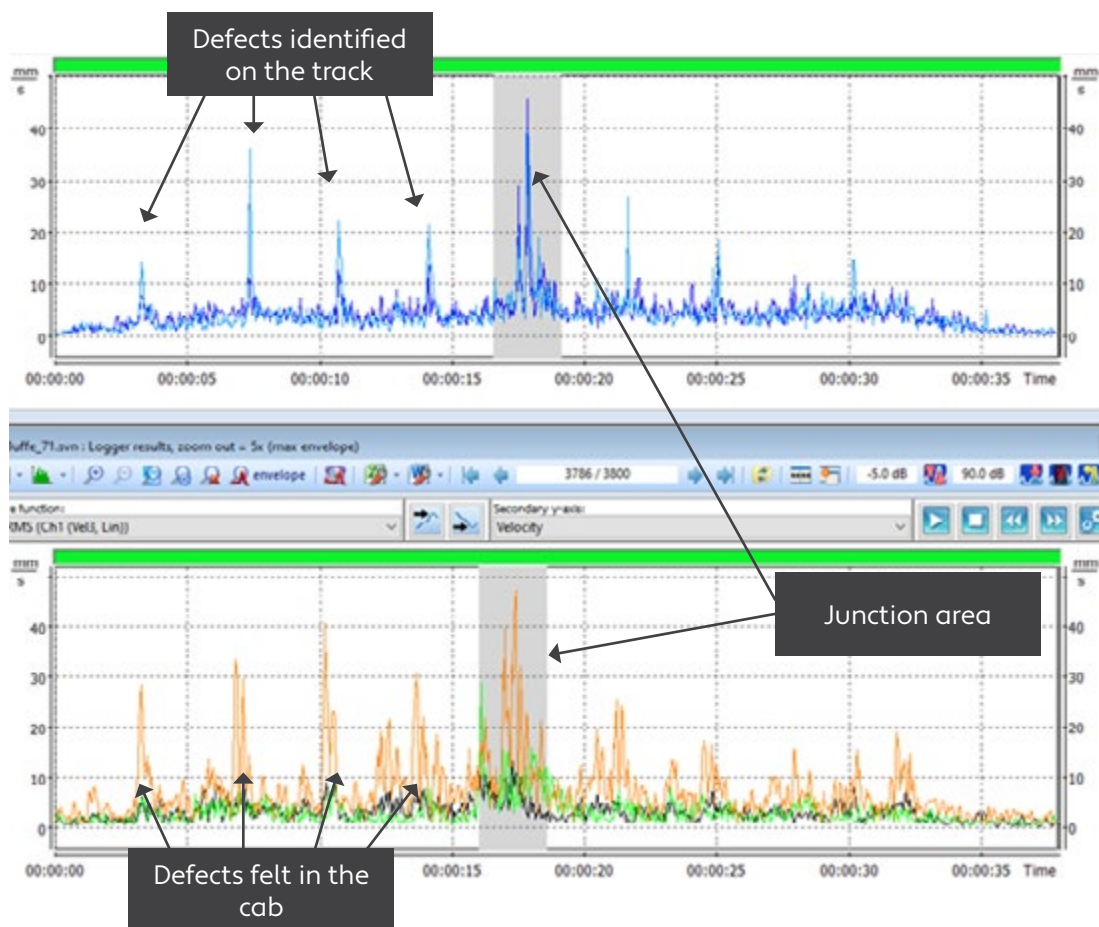
Figure 4 – Above RMS vibration in mm/s measured on the trolley wheels, below RMS vibration in mm/s on the driver seat
